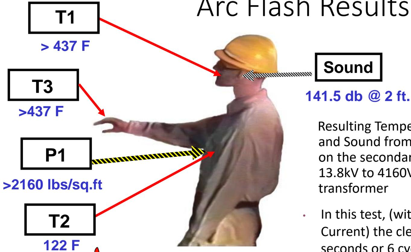
Resulting Temperature, Pressure and Sound from a short circuit on the secondary side of a 13.8kV to 4160V, 10MVA transformer
