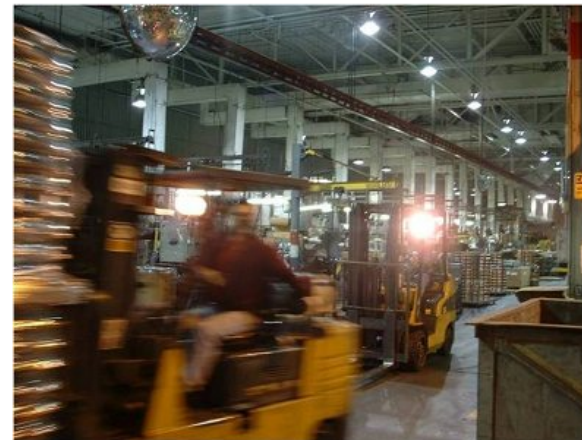
Moving industrial equipment have also been fitted with noise generators and strobe lights.
